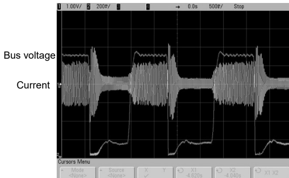
Figure 2 The inverter realizes stable control of current and voltage, no trip under any acceleration and deceleration condition, as well as stable operation condition
